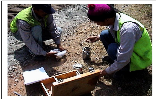
Getting In-situ Moisture Content using Speedy Moisture Tester
